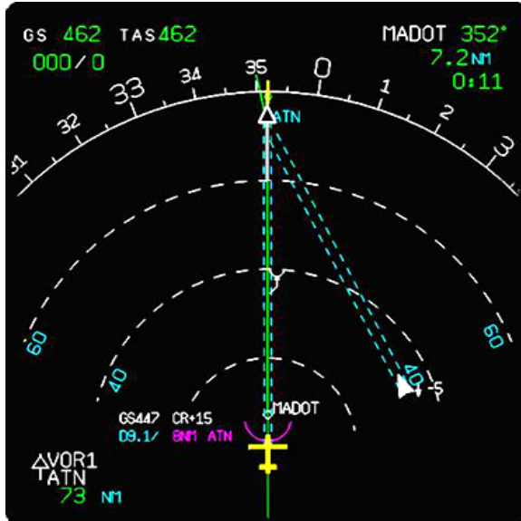
Fig. 3: CDTI screen for Airborne Spacing application.
